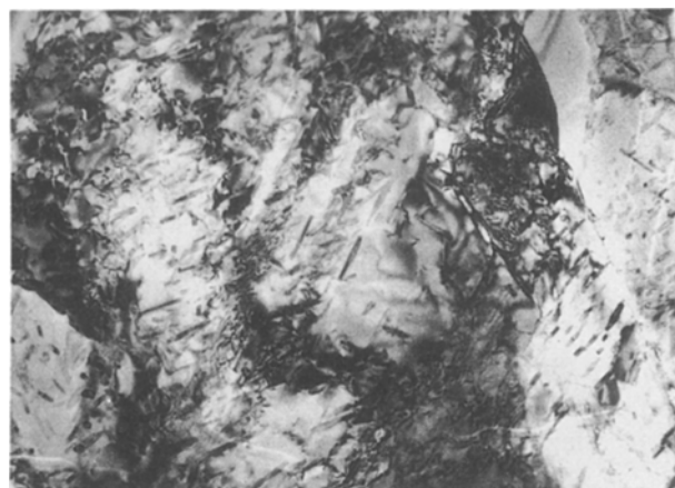
Figure 8 Ferrite structure obtained after quenching aged at 550 °C, + 4 h; \times 36\,000 .
