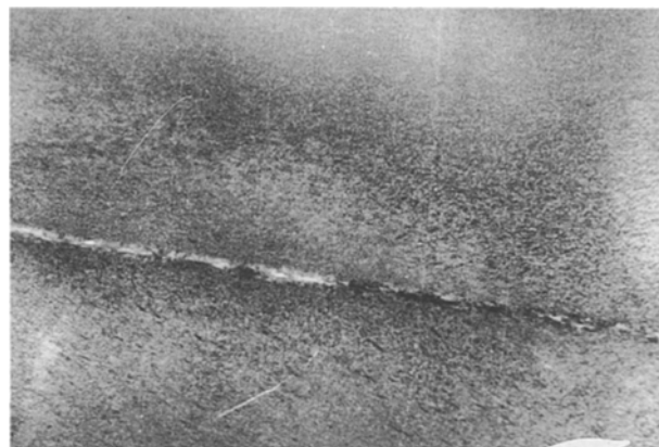
Figure 2 The structure of nitrous austenite after quenching from 1150 °C; \times 36\,000 .
