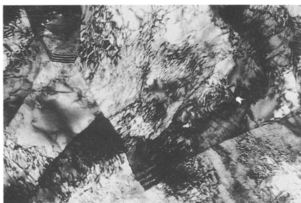
Figure 1 The structure of high-temperature nitrous ferrite after quenching from 900 °C, \times 36\,000 .
